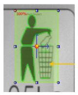
4. Manual removal of meaningless contours: if at end of the noise removal, some meaningless contours are still present, the user can remove them manually. To proceed manually, the user must select each contour to remove with the left mouse button. When aimed, the contour to remove will be highlighted in yellow. When selected, the contour to remove will be represented in red.
