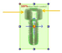
3. Manual removal of meaningless contours: if at end of the noise removal, some meaningless contours are still present, the user can remove them manually. To proceed manually, the user must select each contour to remove with the left mouse button. When aimed, the contour to remove will be highlighted in yellow. When selected, the contour to remove will be represented in red.
