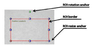
If you want to change the ROI size, left-click and drag one of the blue anchors you find on ROI borders. If you want to move the ROI, place the cursor over one of the 4 ROI borders; it will change its icon into a 4 crossed-arrowed one. Press and hold the left mouse button, and drag the rectangle to the desired position if the image.
