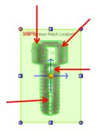
2. Noise removal: contours generated by weaker reflections can be removed using the "Noise Removal" parameter in the Expert panel of the 360° Contour Match locator parameters. In general, the higher the value of this parameter, the lower the number of contours found inside the TEMPLATE ROI.
