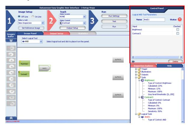
For each Logical Tool, the CONTROL PANEL displays a table with the list of the possible Inputs that can be connected to the Logical Tool. All the Controls, the Locator and the Logical Tools currently inserted in the Inspection can be configured as Inputs for the current
