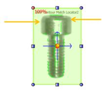
4. Manual removal of meaningless contours: if at end of the noise removal, some meaningless contours are still present, the user can remove them manually. To proceed manually, the user must select each contour to remove with the left mouse button. When aimed, the contour to remove will be highlighted in yellow. When selected, the contour to remove will be represented in red.
