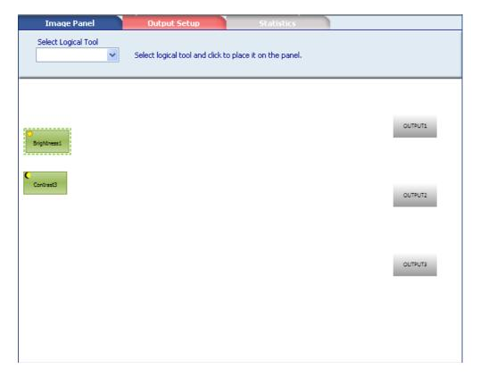
Select the Logical Tool you want to add to the current Inspection using the pull-down menu in the OUTPUT SETUP PANEL under the "Select Logical Tool" label. Once selected, you have
