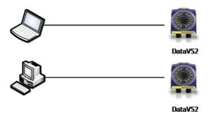
Through LAN: use common network (non-cross) cables normally used to connect devices to routing hubs.
