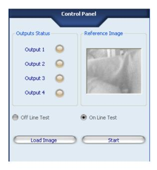
If you are in Offline Mode you can only make an Offline Test: to do so click on the "Load Image" button or click on the IMAGE BUFFER icon in the Tool Bar and select up to 19 images to cycle through for testing.
