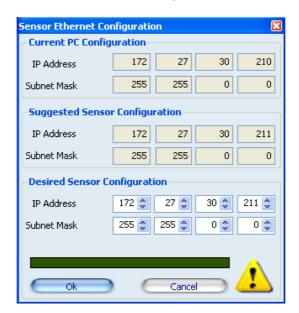
In the top section you find the current IP-Address of the PC. In the middle you find a suggestion on the network settings of the sensor. In the lower section you find the input boxes for the network settings (use arrow keys, numerical entries and the scroll of the mouse-wheel). After clicking on "Ok" the IP-Address will be sent to and stored by the sensor. The new IP-Address will not become active until the next power-up of the sensor.
