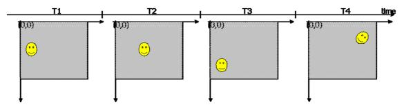
The position of the piece can affect the inspection result and can cause Inspection failure when not necessary (or vice versa), as the sensor doesn't check the right part of the piece. The following figure shows a Brightness Tool execution result: green when it is ok, red when it fails. The Brightness ROI position is fixed and referred to the absolute reference system, while the piece to inspect moves inside it from one image to another.
