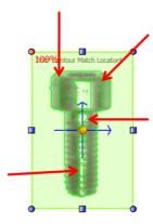
3. Remove noise: contours generated by weaker reflections can be removed using the "Noise Removal" parameter in the Expert panel of the 360° Contour Counter Control parameters. In general, the higher the value of this parameter, the lower the number of contours found inside the TEMPLATE ROI. The following figure shows the effect of this parameter on the example: spurious weaker contours have been eliminated.
