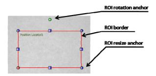
If you want to change the ROI size, left-click and drag one of the blue anchors you find on the ROI borders. If you want to move the ROI, place the cursor over one of the 4 ROI borders; it will change its icon into a 4 crossed-arrowed one. Press and hold the left mouse button and drag the rectangle to the desired position of the image.
