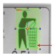
3. Noise removal: contours generated by weaker reflections can be removed using the "Noise Removal" parameter in the Expert panel of the 360° Defect Finder Control parameters. In general, the higher the value of this parameter, the lower the number of contours found inside the TEMPLATE ROI.
