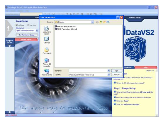
If you choose "Open Inspection from sensor" the DataVS2 GUI opens a dialog. This dialog shows the list of inspections stored on the sensor. Choose one of them and press the "Open" button.
