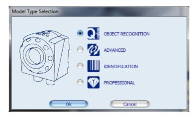
After choosing the Model Type, a File Dialog will be opened by the DataVS2 GUI: this allows you to load the images you want to integrate in your Inspection. You may load more than one image. After you have loaded these images their thumbnails are shown in the IMAGES BUFFER. You can select the current image by simply clicking on the thumbnail. You can load more images by clicking on the "Load Image" button in the CONTROL PANEL.
