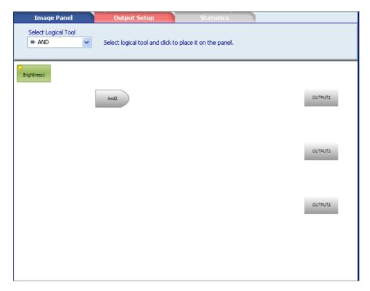
After selecting the Logical Tool, the CONTROL PANEL will display the Logical Tool parameters, represented by the list of all possible Controls that can be connected as inputs to the Logical Tool; the currently connected inputs are shown as checked inputs in the CONTROL PANEL. As soon as the minimum number of Inputs are connected to the Logical Tool, it will change color and become green (SUCCESS) or red (FAILURE) depending on the logical status of the gate.
