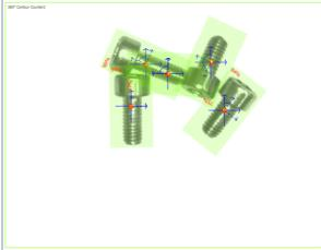
Fig. A Control Contour Counter: Reference Image
