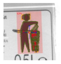
If the object to analyze shows a high defect index, it may not be detected by the 360° Defect Finder Control. In this case, only the SEARCH AREA is displayed in red on the processed image.
