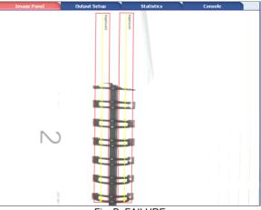
This control is also termed "gauge" and lets you measure the distance between two points (edges).
