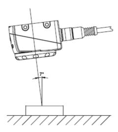
The sensor can be mounted with an angle of 5-7° degrees with respect to the vertical axis of the object; in order to avoid strong reflections from the object.
