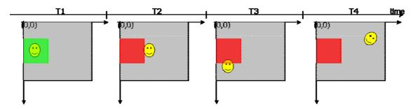
If we desire a reliable behavior we must add a *part finder*, i.e. a locator. With the locator, the image processing cycle is organized in two phases: first the locator searches for the part and returns a position (x,y,alpha), then the Control ROIs are relocated, depending on the current position found by the locator, and Controls are executed. The result of the inspection is successful if both the locator and the controls return a result that satisfies Input conditions.
