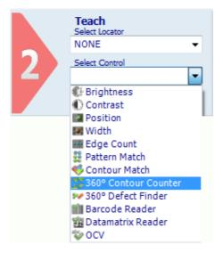
Position the control on the reference image in the IMAGE PANEL: the pointer changes shape as soon as it enters the work area. Left-click once at any position to create a default rectangular ROI.
