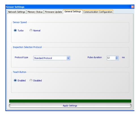
To enable mechanical Teach In function through the DataVS2 GUI, from the Sensor →Settings Menu, open the "General Settings" Tab and in "Teach Button" select the "Enabled" option.
