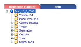
The parameters are displayed in a hierarchic view, where each of them is represented by a branch of the tree.
