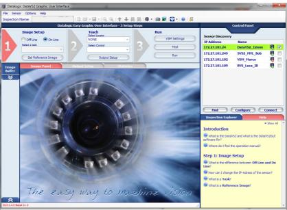
6. Click on the "Connect" button and the software will try to establish a connection with the sensor: if success, a message will appear, displaying the currently connected sensor Model Type and the related Firmware version.
