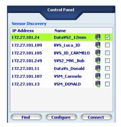
The Control panel shows all sensors found by the Find sensor function. For each sensor the panels shows:
