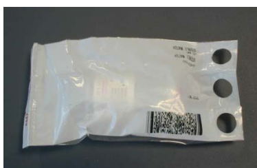
Figure 18 - Unidose Flow-Pack with PDF417 Code
