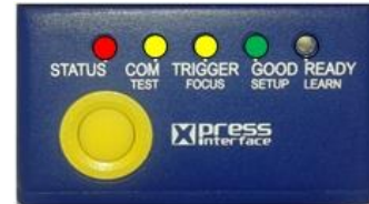
Figure 9 – X-PRESS™ Interface: Setup Function
