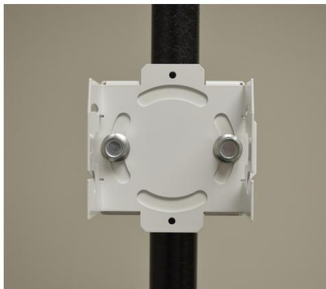
3. Position the Access Point bracket section so that the bottom of the section with the straight (not bevel cut) sides is oriented toward the bottom side of the AP with the gore vent. Using a torque wrench or a ratchet and a 10mm socket, or an adjustable wrench, attach (but don't tighten) the Access Point bracket section to the AP 7161 with the four M6 hex flange screws.
