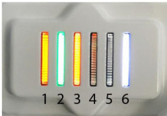
The Access Point utilizes two different colored lights below each LED. Only one light displays within an LED at any given time. Every light within each LED is exercised during startup to allow the user to see if an LED is not functioning. The LEDs turn on and off while rotating in a circular pattern. Since two LEDs feed each light pipe, the pattern is from left to right (LEDs 1 through 6), then right to left (LEDs 6 through 1).
