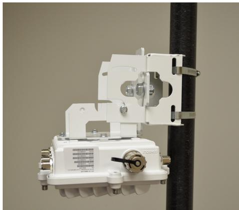
6. Rotate the Access Point bracket section upward and align the top holes on the sides with the top holes on the angle adapter bracket section. Insert two M6 hex flange screws into the top holes on the angle adapter bracket section.
