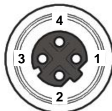
Figure 82 - M12 D-Coded Female Ethernet Network Connector
