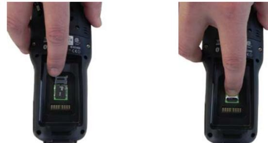
6. Insert the battery's alignment lugs into the recesses, then press firmly until the battery latch clicks twice.
