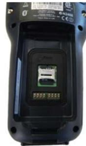
5. Lock the card into place by pushing the cardholder down and then shifting it downwards:
