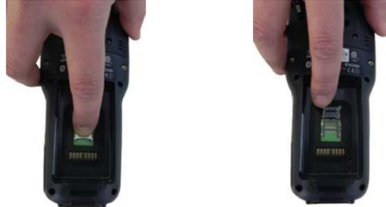
4. Insert the microSD card with the written part upward:
