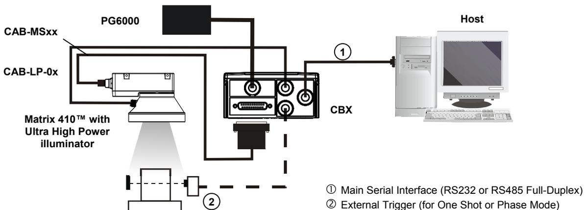
Figure 3 – Matrix 410 655-0x0 Models in Stand Alone Layout
