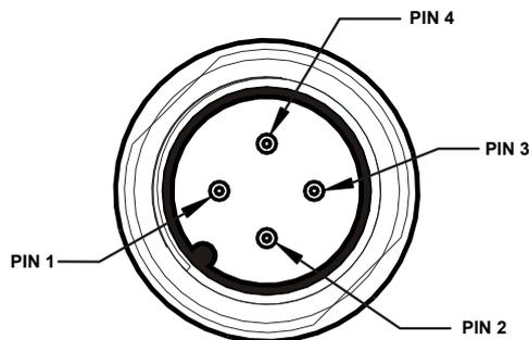
Figure 80 - M12 4-pin Male Ultra High Power Illuminator Input Power Connector
