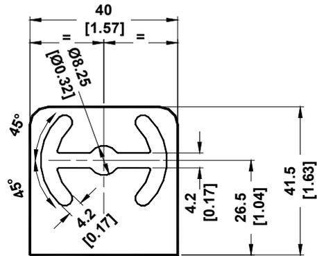
Figure 45 - Mounting Bracket Overall Dimensions
