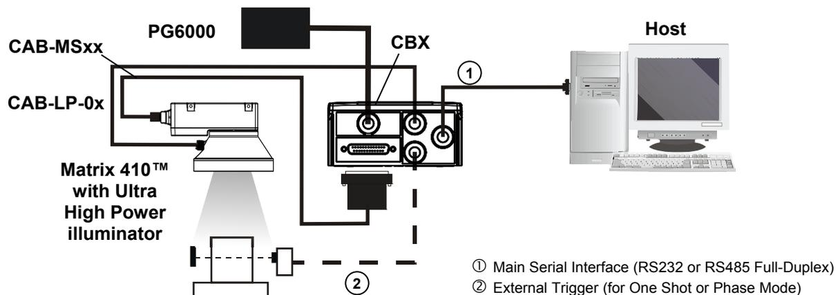
Figure 106 – Serial Interface Point-to-Point Layout
