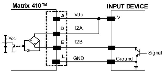
Figure 99 - Input NPN Using Matrix 410™ Power
