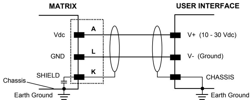
Figure 79 - Power Supply Connection
