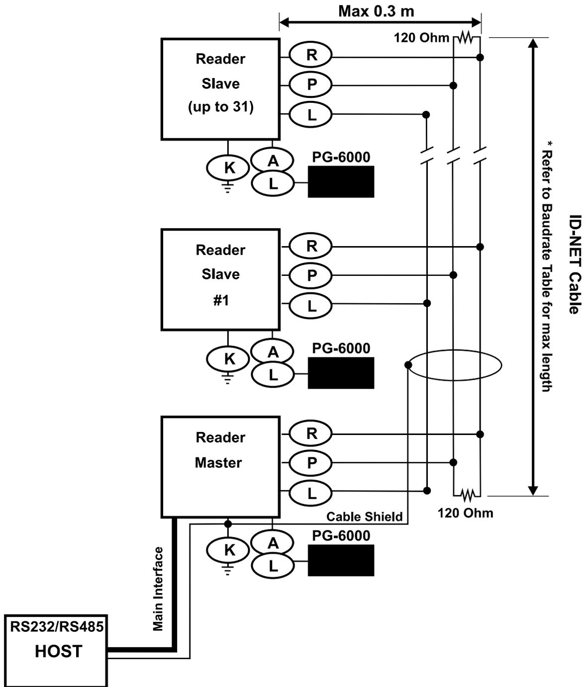
Figure 88 – ID-NET™ Network Connections with isolated power blocks
