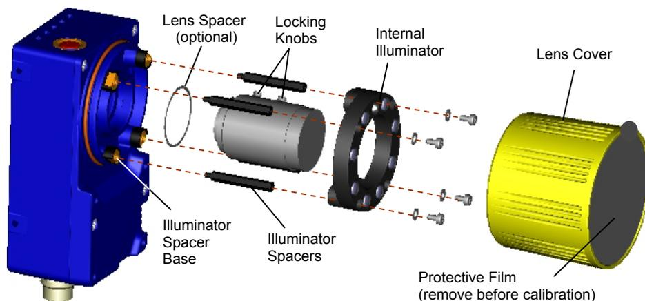
**Figure 1 – Assembling Matrix 410™ Accessories**
