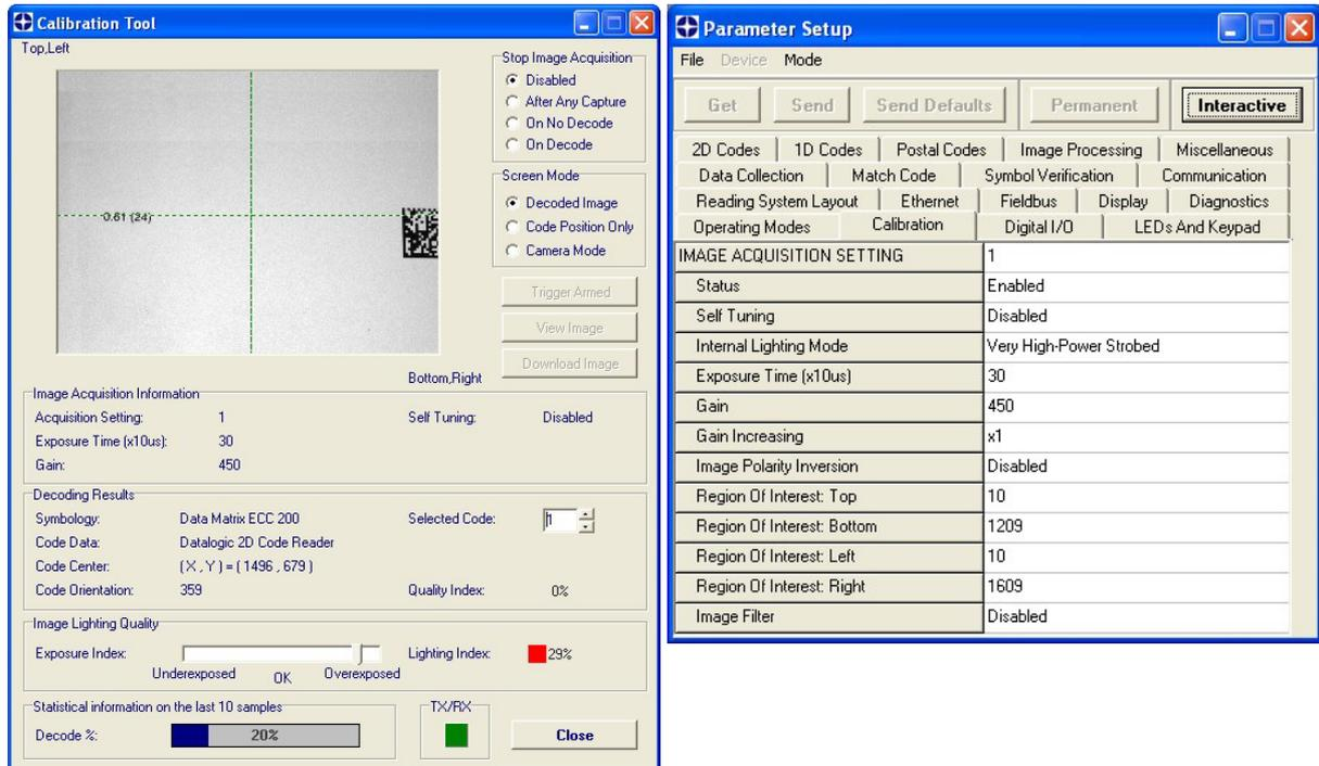
Figure 133 - Example out of FOV
