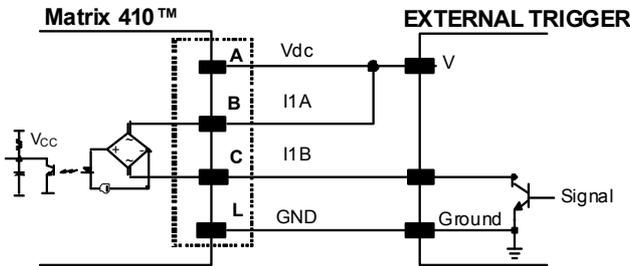
Figure 95 - External Trigger NPN Using Matrix 410™ Power
