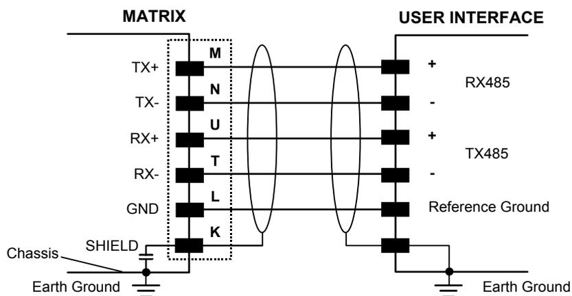
Figure 83 - RS485 Full-duplex Connections
