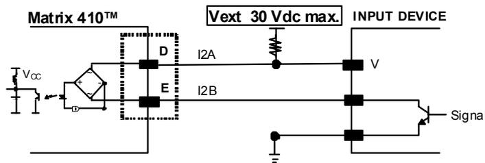
**Figure 101 - Input NPN Using External Power**
