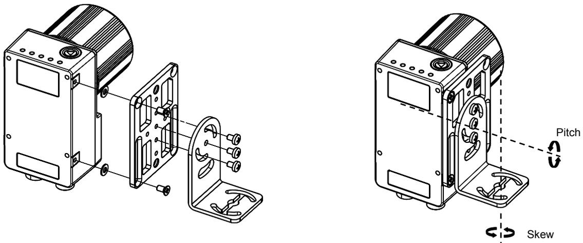
Figure 47 –Positioning with Mounting Bracket (Side)
