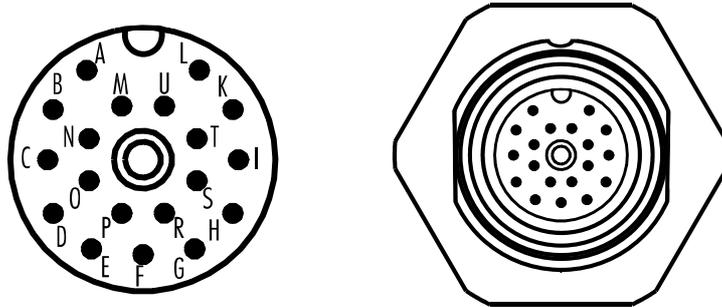
Figure 77 – M16 19-pin Male Connector
