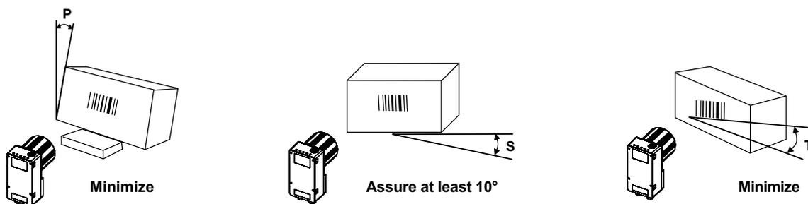
Figure 6 – Pitch, Skew and Tilt Angles
