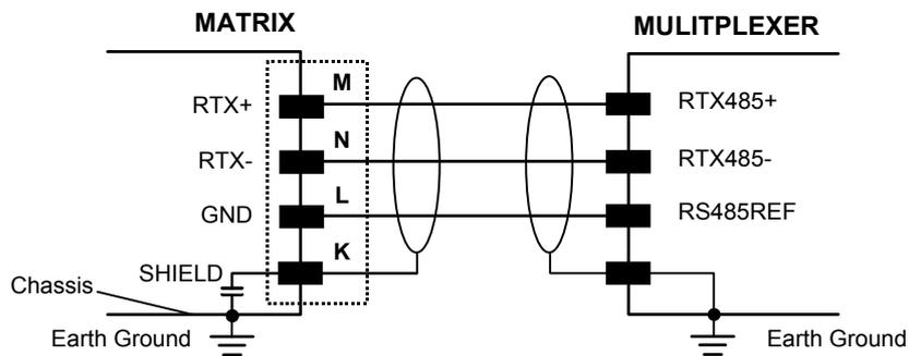
**Figure 85 - RS485 Half-duplex Connections**
