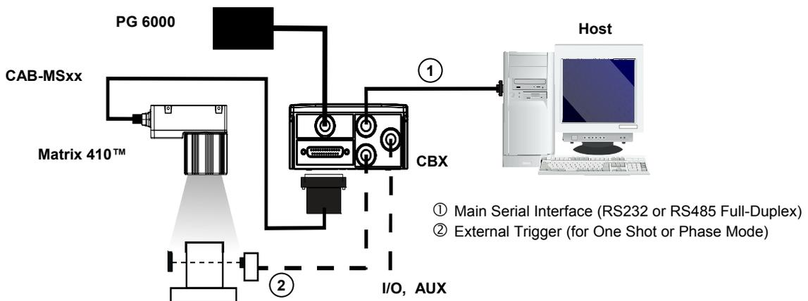
Figure 2 – Matrix 410™ in Stand Alone Layout
