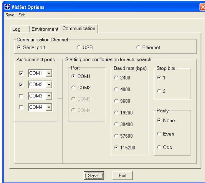
Figure 127 - Options – Communication: Serial Port
