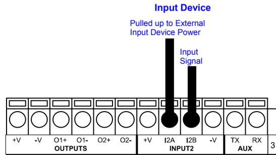
Figure 71 - NPN Input 2 Using External Power
