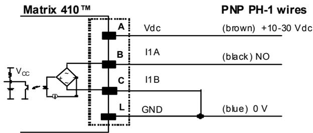
Figure 93 - External Trigger Using PNP PH-1 Photocell
