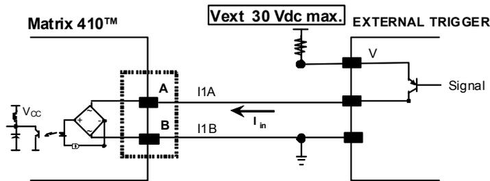
Figure 96 - External Trigger PNP Using External Power
