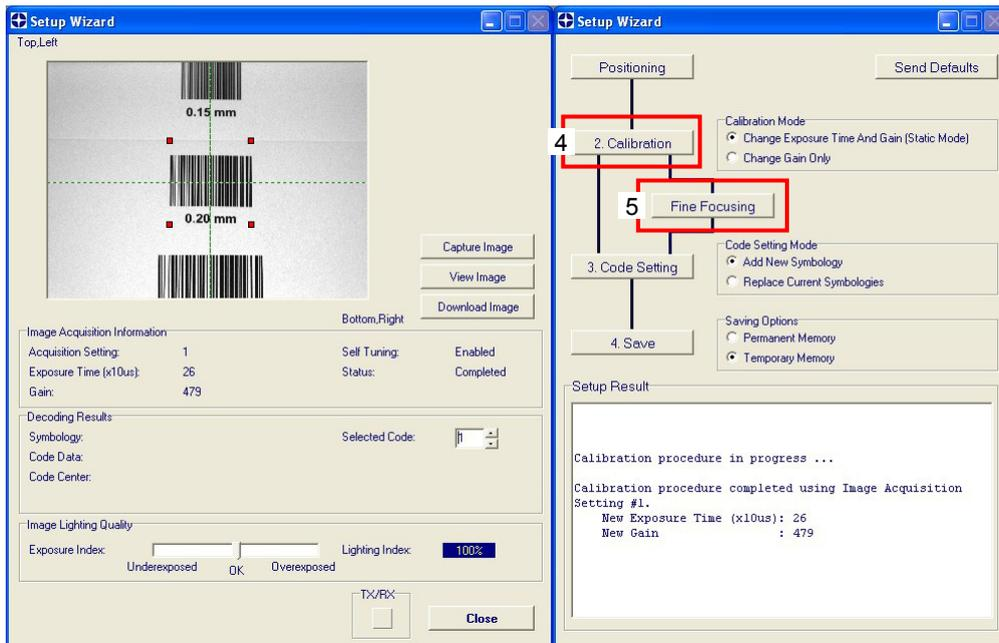
5. Press the "Fine Focusing" button to activate the Fine Focusing Tool. The reader continuously acquires images and gives visual feedback on the focusing quality in the Focusing Tool window.
