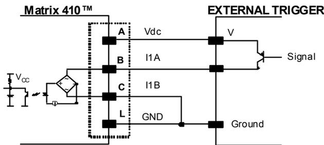
Figure 94 – External Trigger PNP Using Matrix 410™ Power
