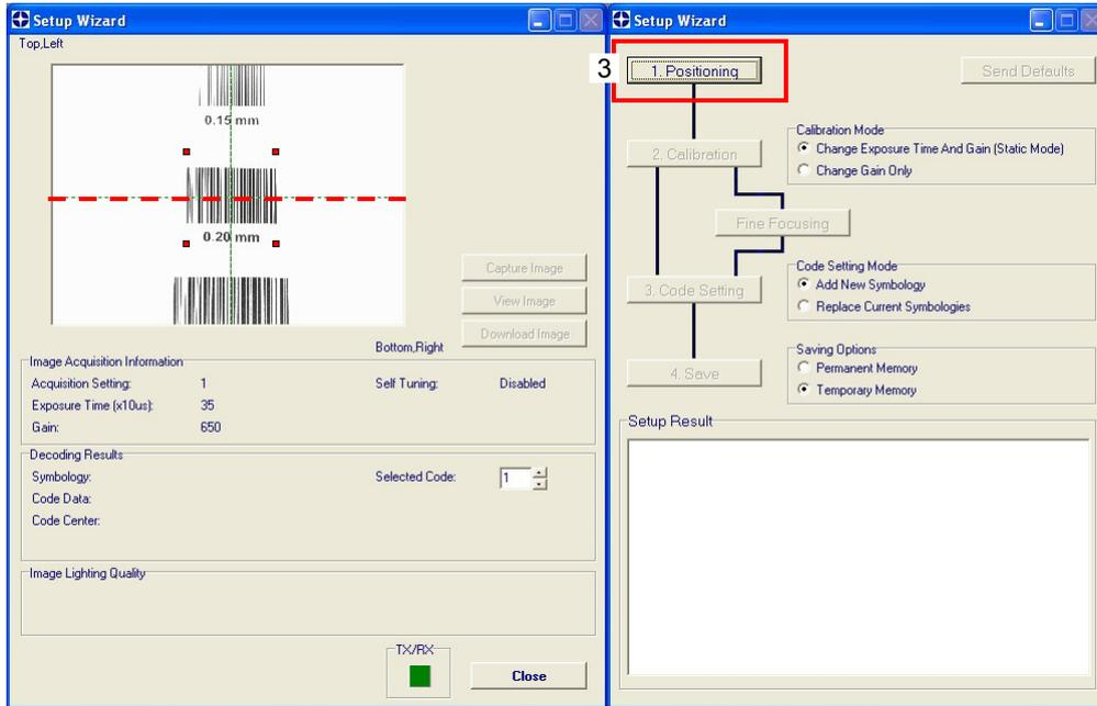
4. Select a Calibration Mode choice and press the "Calibrate" button. The reader flashes once acquiring the image and auto determines the best exposure and gain settings. If the code symbology is enabled by default, the code will also be decoded.
