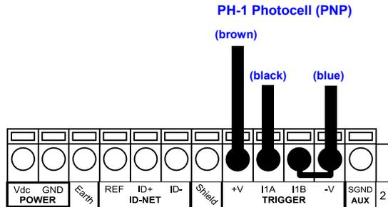
**Figure 66 – PH-1 External Trigger Using MATRIX 410™ Power**
