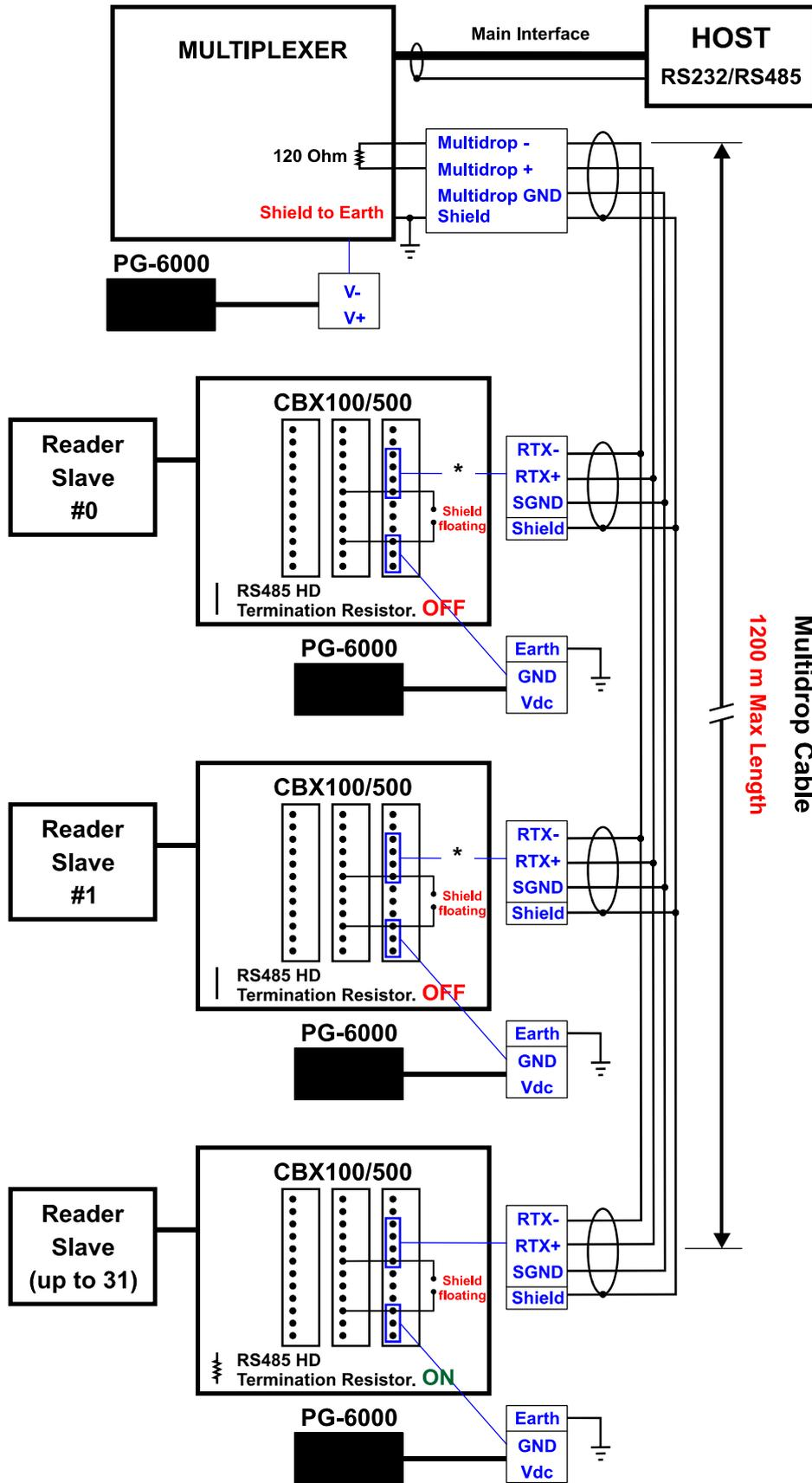
Figure 59 - Matrix 410™ Multidrop Connection to a Multiplexer
