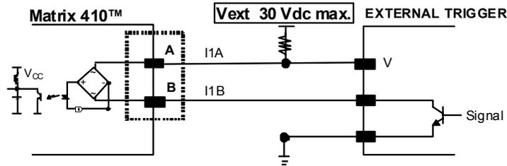
Figure 97 - External Trigger NPN Using External Power
