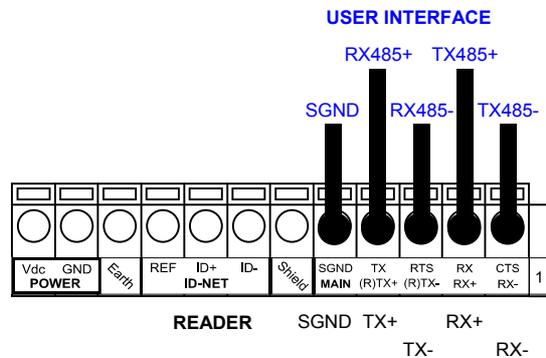
Figure 56 - RS485 Full-duplex Connections
