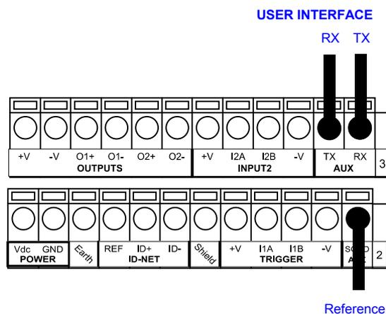
Figure 65 - RS232 Auxiliary Interface Connections
