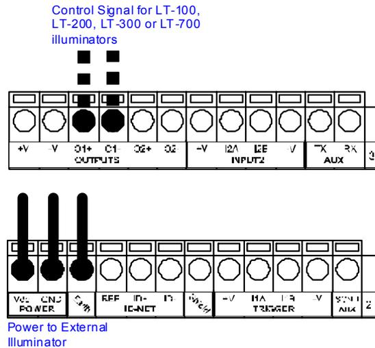
Figure 76 – External Lighting System Connections
