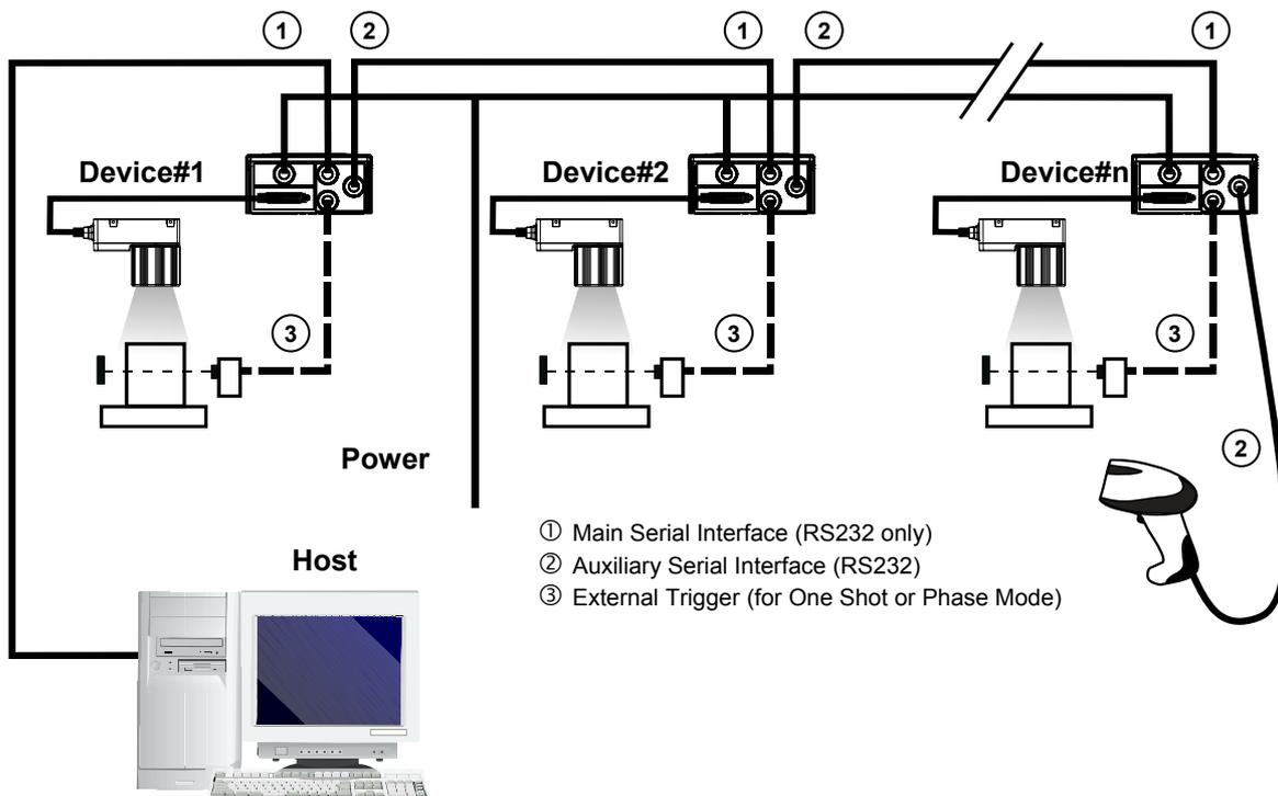
Figure 109 – Pass-Through Layout
