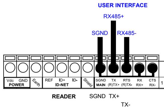
Figure 57 - RS485 Full-duplex Connections using Only TX Signals
