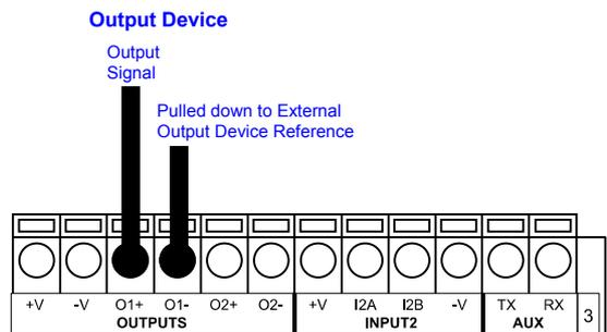
**Figure 75 - Output Open Collector Using External Power**
