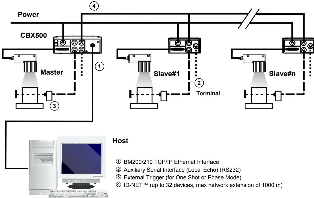
Figure 116 – ID-NET™ M/S Multidata Layout with BM200/210 TCP/IP Ethernet Interface to Host
