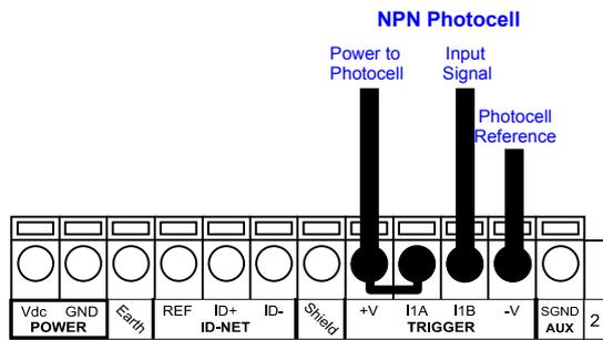
**Figure 67 - NPN External Trigger Using MATRIX 410™ Power**
