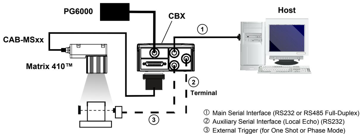
Figure 105 – Serial Interface Point-to-Point Layout
