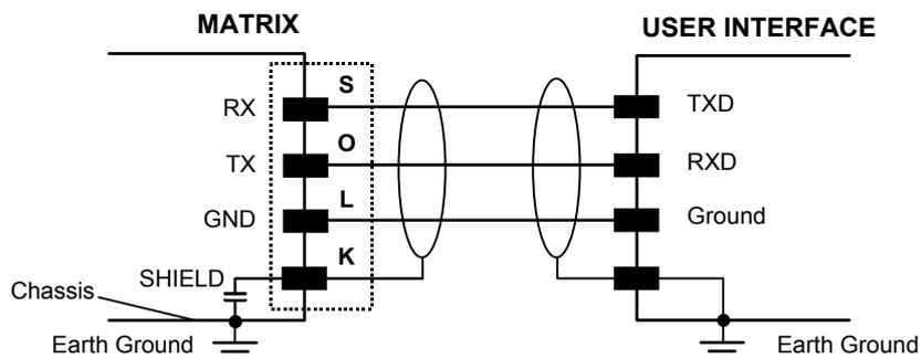
Figure 91 - RS232 Auxiliary Interface Connections Using 19-pin Connector
