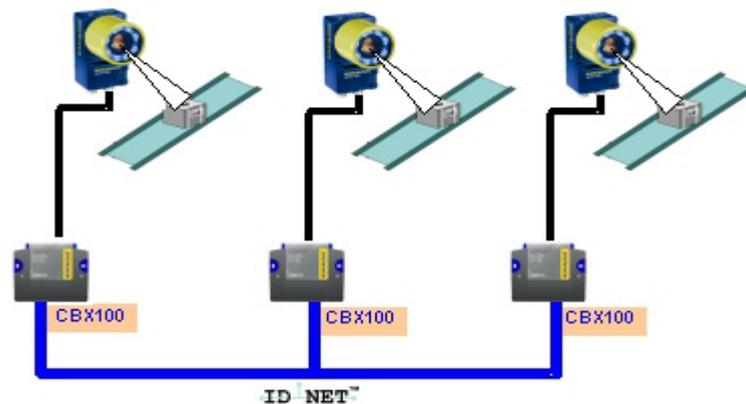
ID-NET™ interface allows connection of readers reading objects placed on independent conveyors. All readers are typically located far away from each other and they use a dedicated presence sensor.
