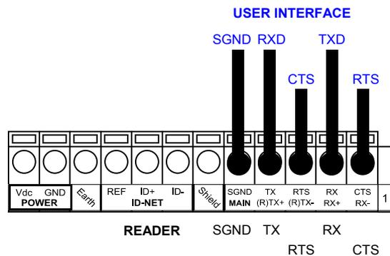
Figure 54 – RS232 Main Interface Connections Using Hardware Handshaking
