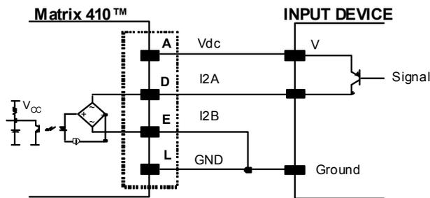
Figure 98 - Input PNP Using Matrix 410™ Power
