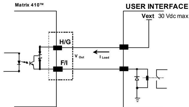
Figure 102 - Open Emitter Output Connection
