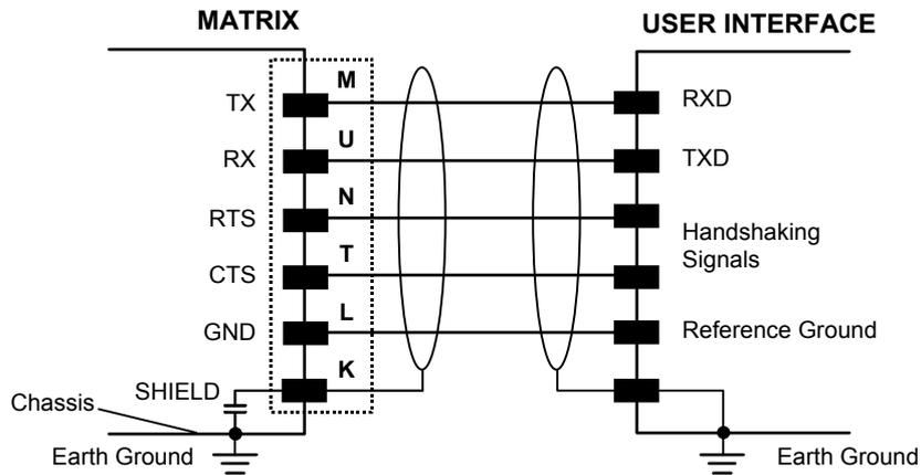
Figure 81 - RS232 Main Interface Connections
