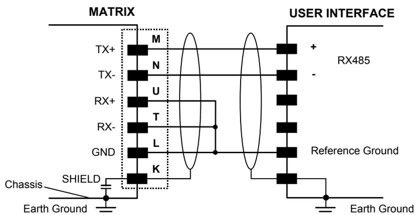
Figure 84 - RS485 Full-duplex Connections using Only TX Signals
