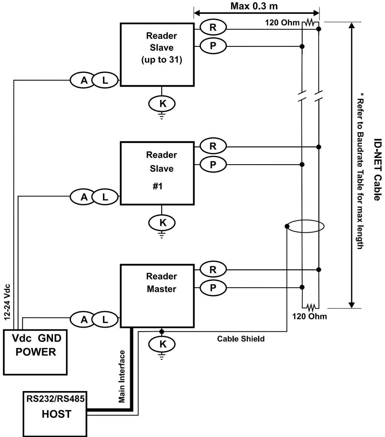
Figure 90 – ID-NET™ Network Connections with Common Power Star Network
