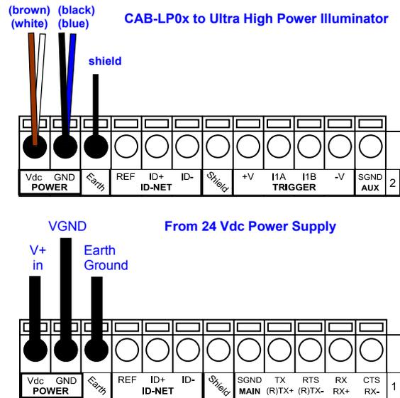
Figure 53 - Power Supply Connections for Matrix 410 655-0x0 Models
