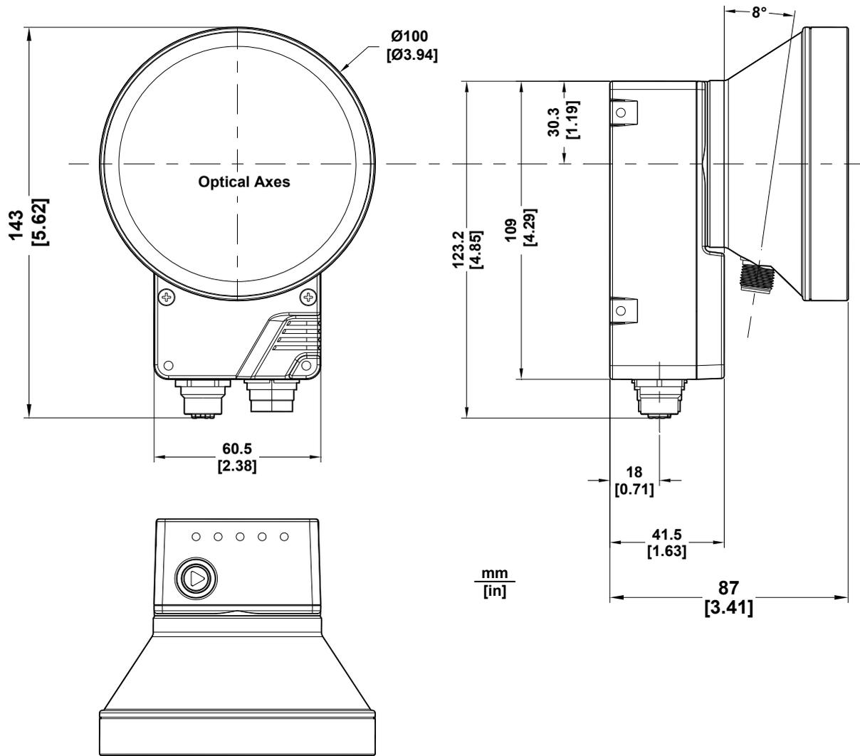
Figure 44 - Matrix 410 655-0x0 Model Overall Dimensions
