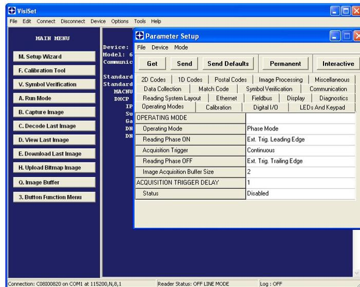
Figure 19 - VisiSet™ Parameter Setup Window
