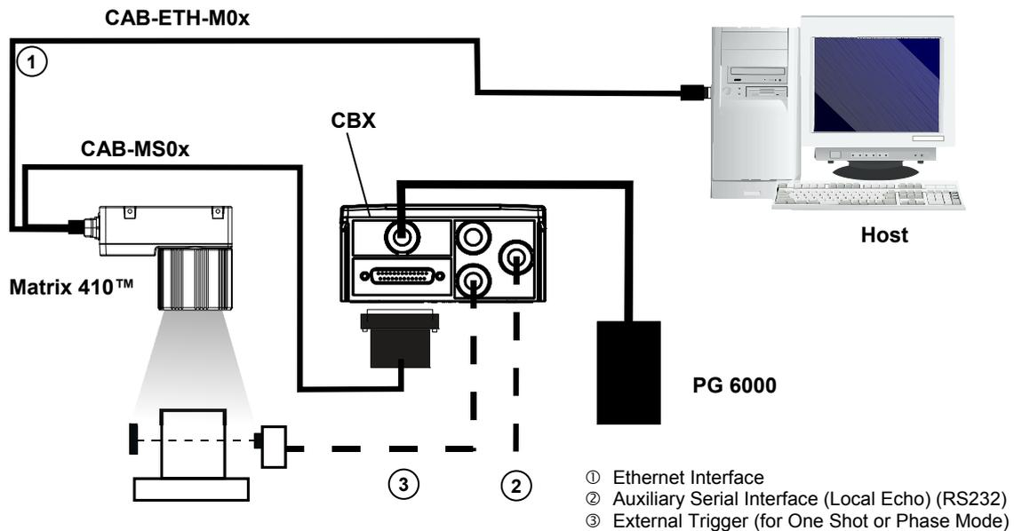
Figure 121 - Ethernet Point-to-Point Layout
