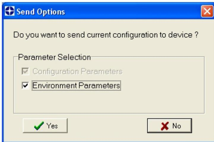
In order to return a device to its absolute default parameters including Environmental parameters, the following "Send Default Configuration with Options" dialog must be used:
