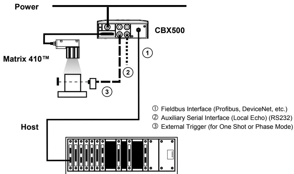
Figure 108 – Fieldbus Interface Point-to-Point Layout
