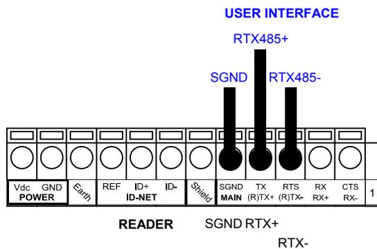
**Figure 58 - RS485 Half-duplex Connections**
