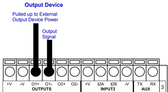
**Figure 74 - Output Open Emitter Using External Power**
