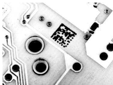
**Figure 29 - Data Matrix Code Directly Marked on PCB Surface by Using Laser Etching Technology**
