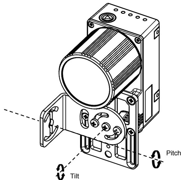
Figure 48 –Positioning with Mounting Bracket (Front)
