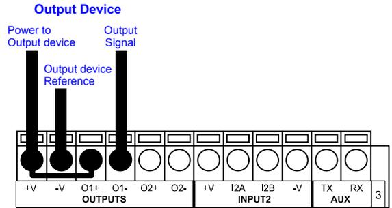
**Figure 72 - Open Emitter Output Using MATRIX 410™ Power**
