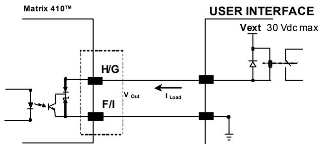
Figure 103 - Open Collector Output Connection
