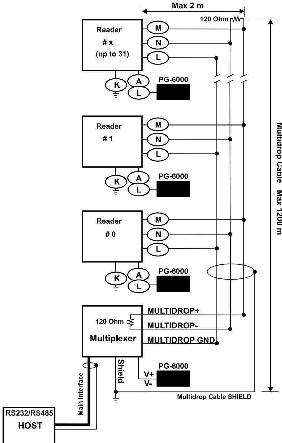
Figure 86 - Matrix 410™ Multidrop Connection to a Mutiplexer
