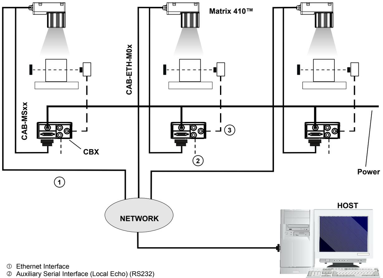
Figure 122 - Ethernet Network Layout
