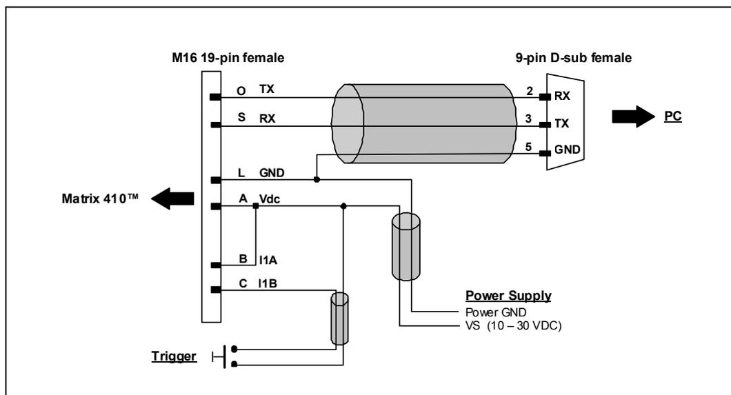
Figure 104- Test Cable for Matrix 410™
