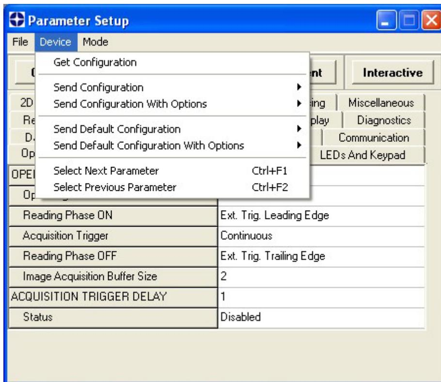
Environmental Parameters regard the device Identity and Position in a Network (ID-NET™, Master/Slave RS232, MUX 32, Ethernet) and are not influenced by the "Send Default Configuration" and "Send Configuration" commands. This allows individual devices to be configured differently without affecting their recognized position in the network.
