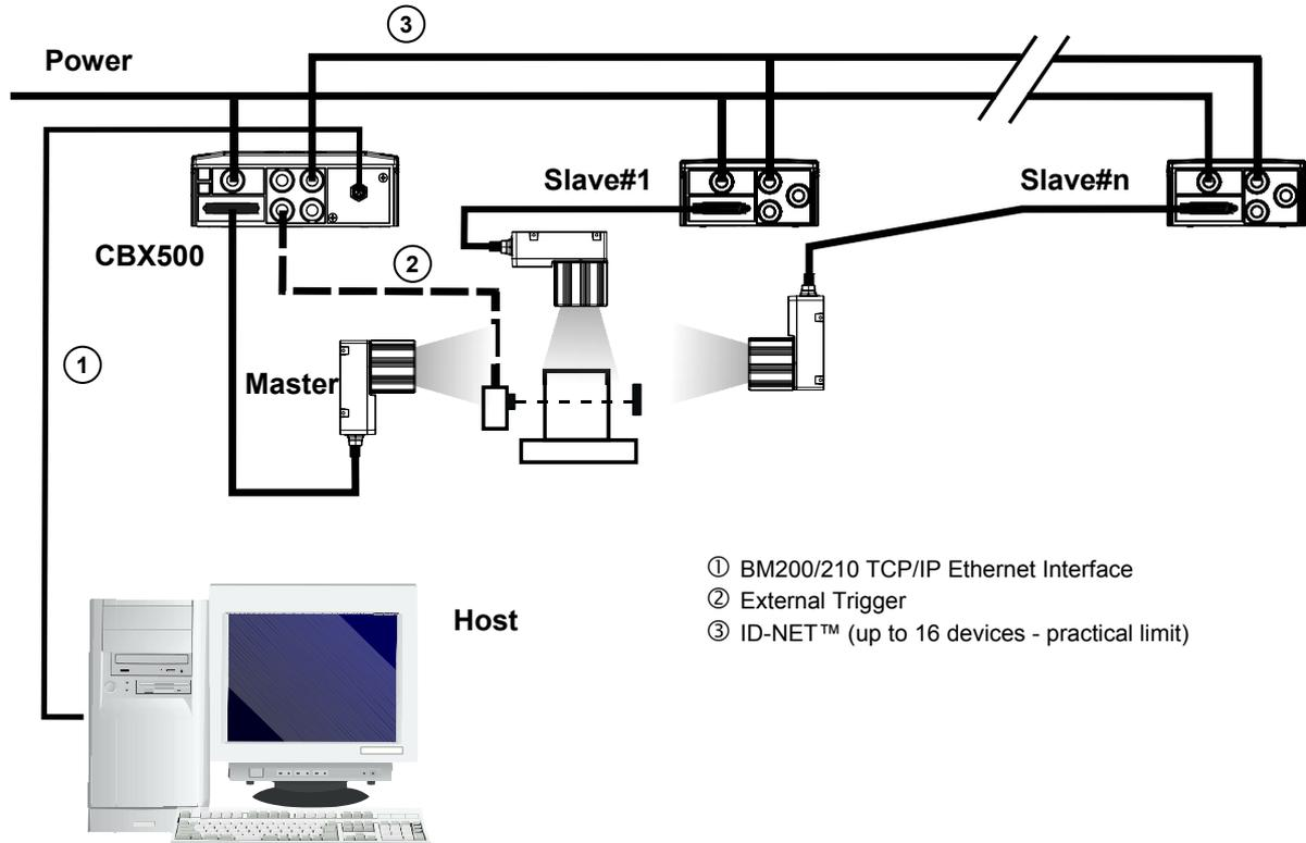
Figure 114 – ID-NET™ M/S Synchronized Layout with BM200/210 TCP/IP Ethernet Interface to Host
