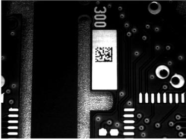
Figure 30 - Dot Matrix Code Directly Marked on PCB Copper Pad by Using Ink-Jet Technology
