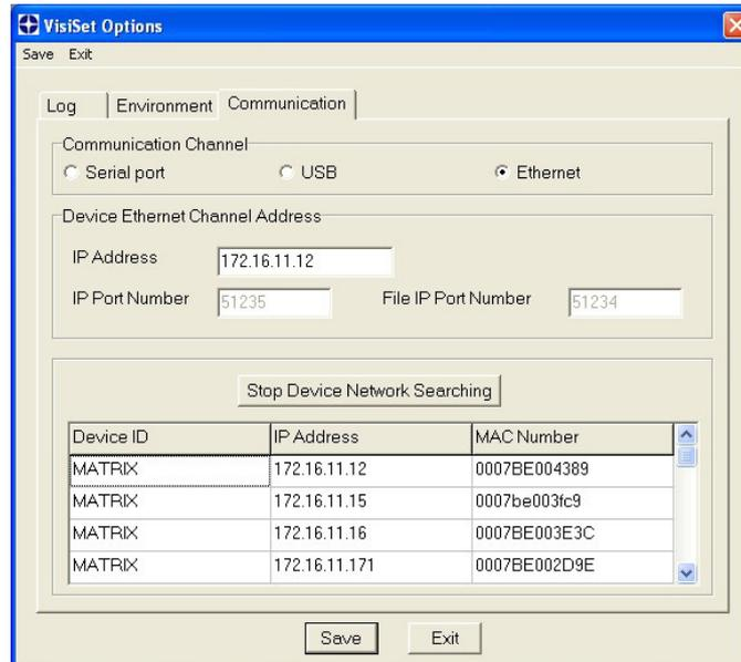
Figure 128 - Options – Communication: Ethernet
