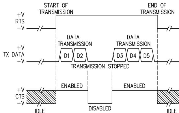
Figure 82 - RS232 Control Signals
