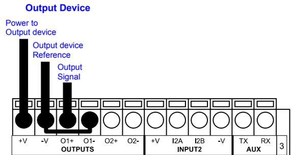
**Figure 73 - Open Collector Output Using MATRIX 410™ Power**
