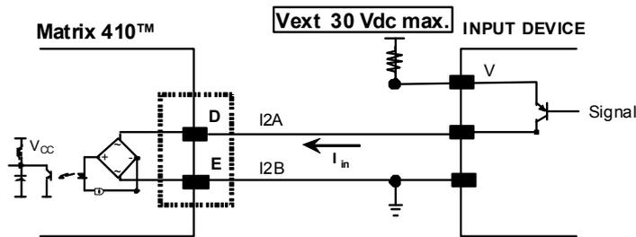
**Figure 100 - Input PNP Using External Power**
