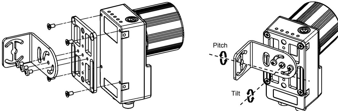
Figure 46 –Positioning with Mounting Bracket (Back)
