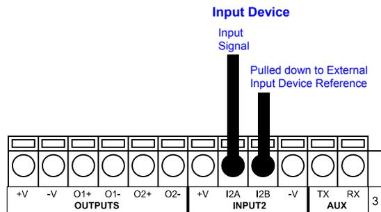
**Figure 70 - PNP Input 2 Using External Power**
