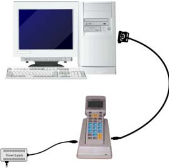
Figure 17 - Downloading Data with F734-E
